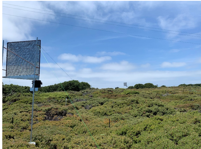
Figure 23. Three 1-meter fog collectors arranged in a transect up a slope in rare maritime chaparral habitat at FONR.
