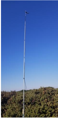
ACOUSTIC BAT MONITORING STATION
