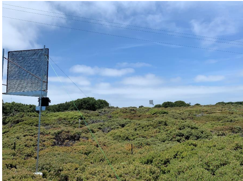
Figure 17. Three 1-meter fog collectors arranged in a transect up a slope in rare maritime chaparral habitat at FONR.
